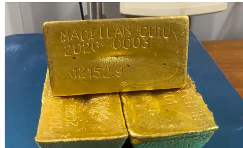
Gold dore resulting from commissioning process containing 1,130oz of gold
