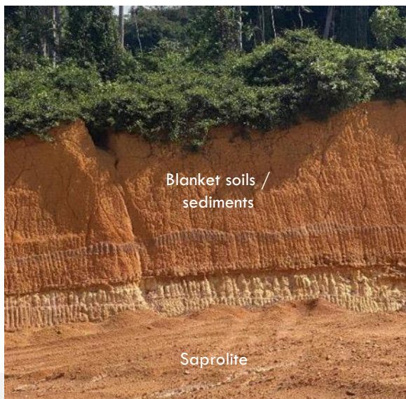
Section through mineralized gold-in-oxide material at Cuiu Cuiu showing blanket soils and sediments overlying saprolite (weathered bedrock)
