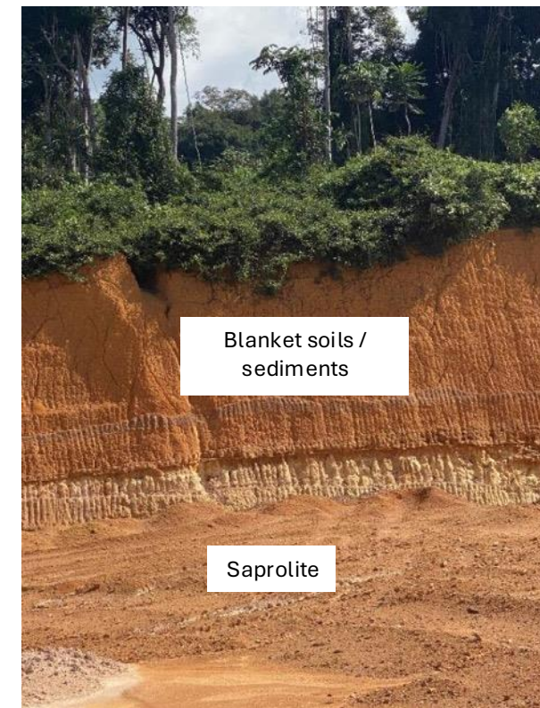
Section through mineralized gold-in-oxide material at Cuiu Cuiu showing blanket soils and sediments overlying saprolite (weathered bedrock)
