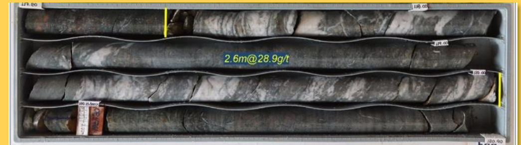
High-grade zone in DDH271 which returned 2.6m @ 28.9 g/t gold including 1m @ 64.6 g/t gold
